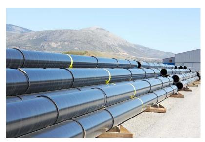
The agreement covers approximately 76km of 8" - 16" High Frequency Welded (HFW) linepipe which will include external 3-layer polyethylene coating. The HFW pipes will be manufactured and coated at Corinth's facility in Greece and delivered directly to Mozambique within 2022.
