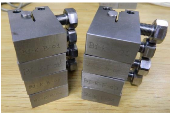
Figure 1: Fracture toughness specimens used in high pressure hydrogen testing
