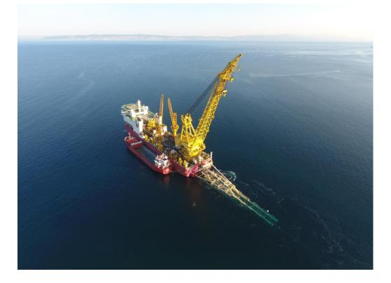
Corinth Pipeworks supplied 37Km of DNV SAWL 450FD 36" pipes with 3LPE anticorrosion coating and concrete weight coating for the TANAP offshore pipeline to SapuraEnergy, a leading global integrated oil and gas services and solutions provider operating across the entire upstream value chain.
