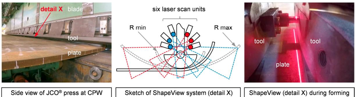
Fig. 3. ShapeView system integrated into the blade during forming
