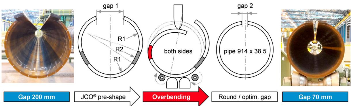
Fig 2. Pipe closing process with special pre-shape
