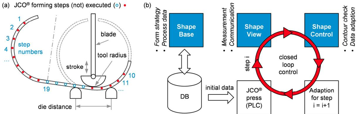
Fig. 1. JCO<sup>®</sup> forming process (a), interaction of the Shape modules for process control (b)
