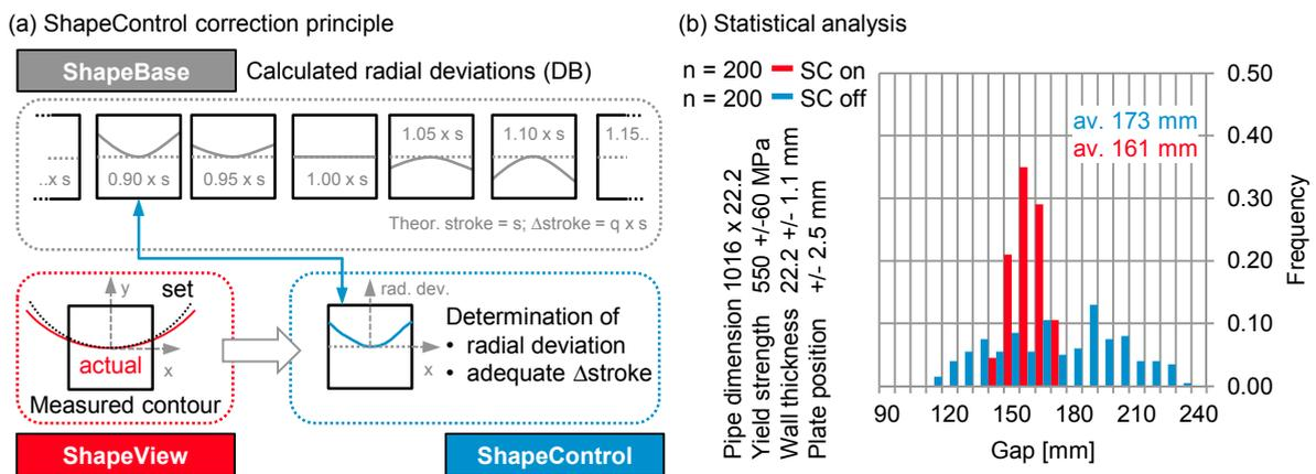
Fig. 4. ShapeControl (SC) principle (a), effects of ShapeControl on gap via statistical analysis (b)
