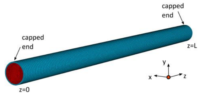
Fig. 10 Three-dimensional finite element model of pipe specimens
