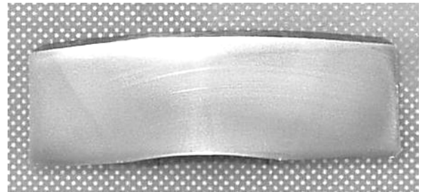
Figure 14: Pipe after double normalizing with intermediate cooling
